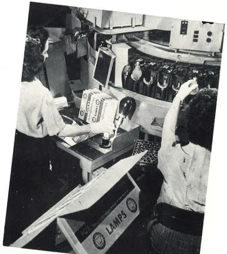
Automatic "Sealex" machines like this one at the Bloomfield, N. J., plant exhaust and seal incandescent light bulbs. One machine is capable of turning out 9,000 bulbs on just one shift.
