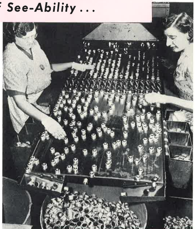
Bases for incandescent lamps are turned out by automatic machines like this at the Belleville, N. J., plant.
