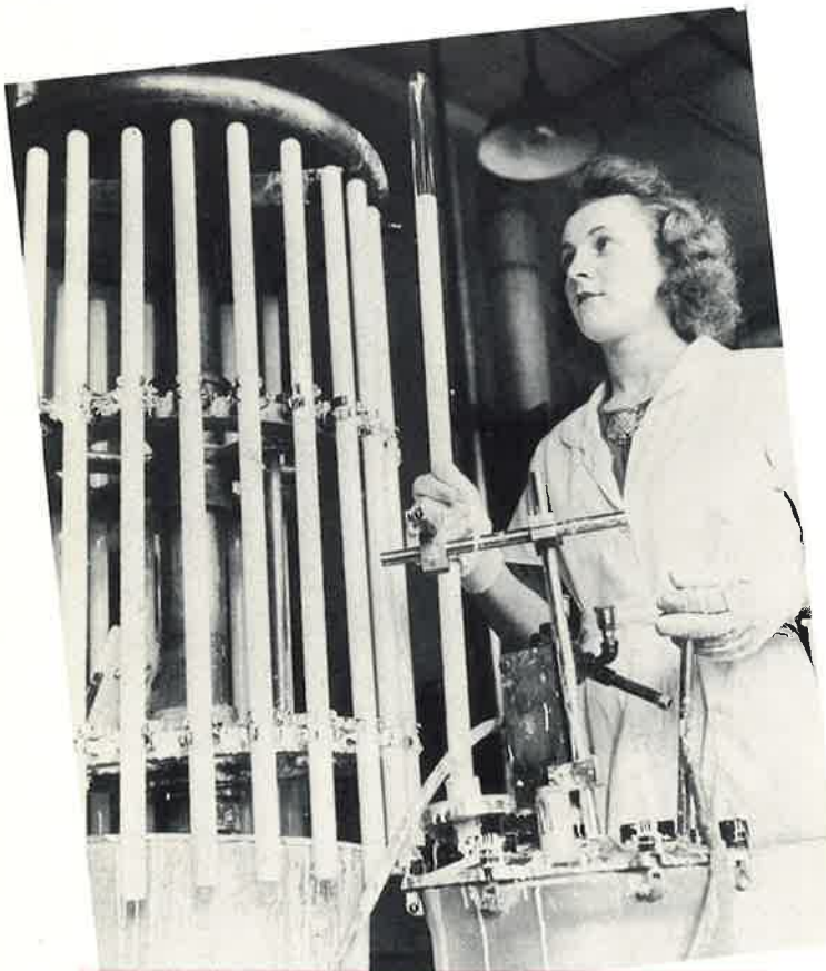
Tubes of glass soon to become fluorescent lamps are coated with light-producing phosphors.
